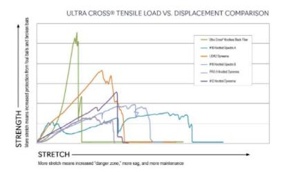
60K 50K 40K 30K 20K 10K 0K #18 knotted #18 knotted Pro-9 knotted #12 knotted UDR2 knotted Litra Cross® Spectra A Spectra B braided /
